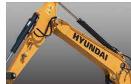
Standard breaker piping
